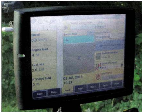
Using an RTK signal, the tractor's terminal is used for guidance.
